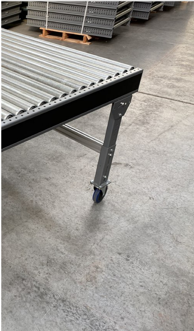
Mobile gravity conveyor with adjustable height legs and lockable casters
