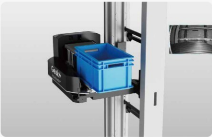
3D camera adaptive tote positioning
